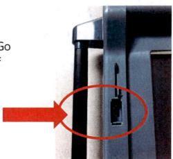
5. Unlock the back panel on the Duo Go carrier and open the back panel door (removing the tamper seal first, if applicable).
