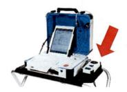
6. Open the Verity Duo case and lock the lid brace in place. ▶
