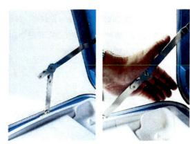
8. Unlock (A), unlatch (B), and remove (C) the tablet. ▼
