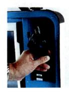
6. Plug the power cord into the power brick, and then plug the power brick into the back of the Verity Scan (flat side up). ▼
