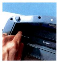
7. Connect the USB cable on the inside of the Duo Go carrier to the port on the side of the tablet. A tamper seal may be used to secure the cable; remove this seal first, if applicable.
