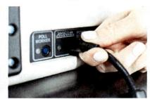
5. If the Duo will be used with Verity Access, connect the Verity Access device now. Connect the blue cord from the Verity Access into the corresponding port on the back of the Duo device. The Access device may be placed in the cradle to the right of the Duo. ▼
