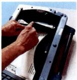
Insert one sheet of thermal paper. Once the paper has fed into the printer, lay the sheet flat as shown.
