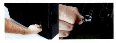
7. Pull the string on the underside of the lid upward to unlock the lid latch.
