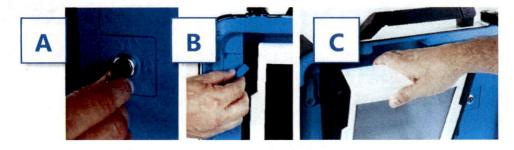
8. Seat the tablet in the cradle (A), tilt it back (B), and lock it in place (C). ▼
