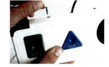
Plug the tactile switches, sip-and-puff, or any other dual-switch input device into the port on the top right of the Verity Access.
