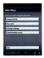
On both Verity Duo and Verity Scan, enter the Suspend Polls Code and select Accept. The Suspend Polls reports will print automatically.
